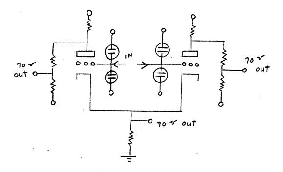
Minor feedback for stability goes through the circuit without changing the neon bulbs. Major feedback for ultrastability changes the neon bulbs, and hence the effective connection of the circuit.
